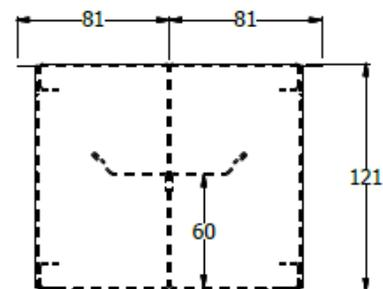
CANALETA CONDUCTORA DOBLE A SUPERFICIE 12X12 LONGITUD 1,00 ( VER CÓDIGO E8-71938-021)
