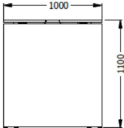
MESA BARRA ESP. H:1.10X3,60X1,00 - MELAMINA - DUCTO CABLEADO CON ESCOBILLA
